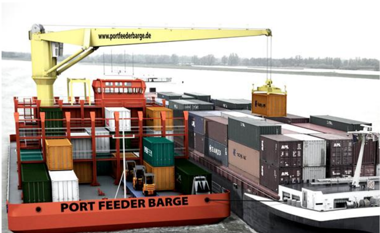
Port Feeder Barge employed as a 'floating terminal' for inland navigation
